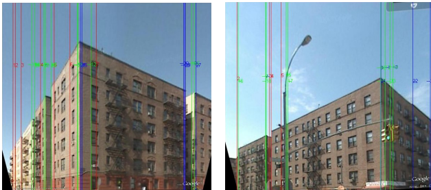
Figure 8. Rectified images with overlay VCLHs.
