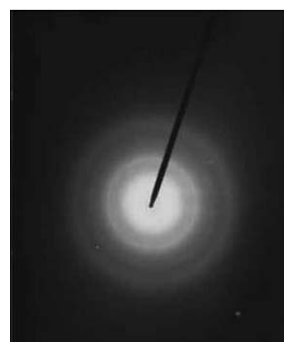
Fig. 3. (a) Typical TEM image of the tip region of a linear-shaped CNF grown on the C/Ni mesh. (b) Electron diffraction pattern taken at the CNF tip.
